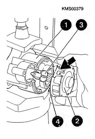
Assembling overrunning-clutch drive and planetary gear train
